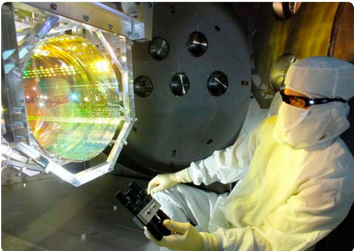
Inspecting the LIGO mirrors (Credit: LIGO)
