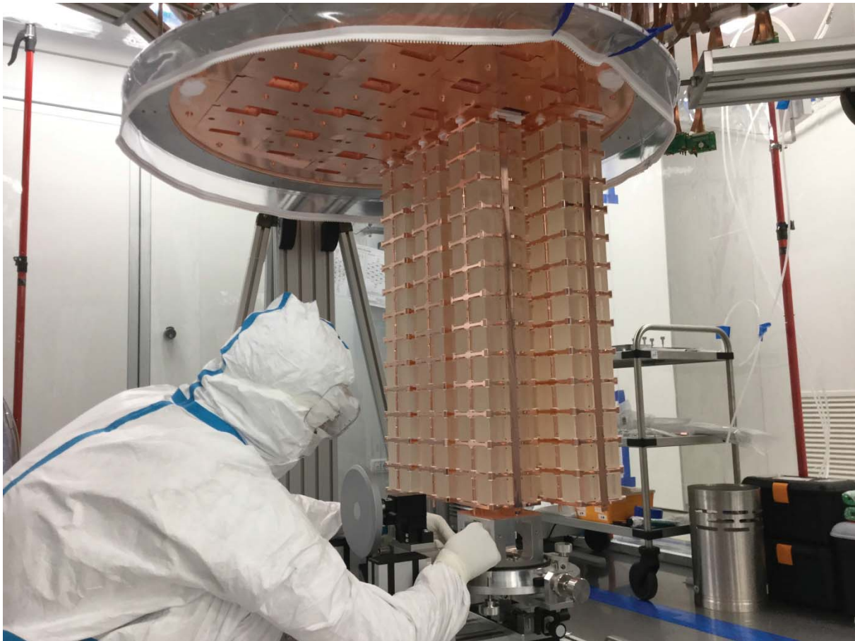
A CUORE engineer operates a custom-built cart to position a tower under the cryostat (CUORE)
