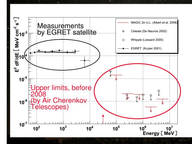
No detection of pulsed VHE gamma rays from Crab before 2008.
