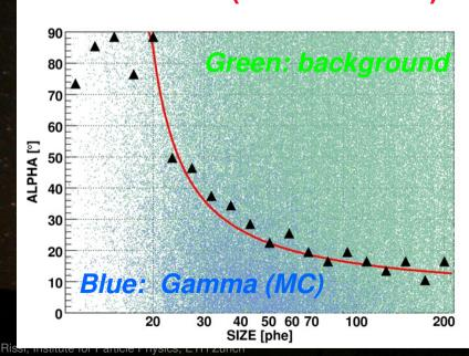
The energy was estimated using the parameter SIZE ( $\sim$  number of Cherenkov photons produced by the  $\gamma$ -ray shower)
