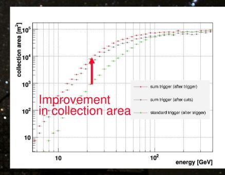
Trigger threshold lowered from 55.GeV to 25 GeV
